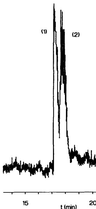
Fig. 3. CE-MS of the stereoisomers EPI (1) and DOX (2) (250 \mu\text{g}/\text{ml} each) in 10 mmol/l sodium acetate buffer (pH 7.5) and 60% methanol using a 700 \times 0.040 mm I.D. capillary and a voltage of 20 kV at the anodic end.
